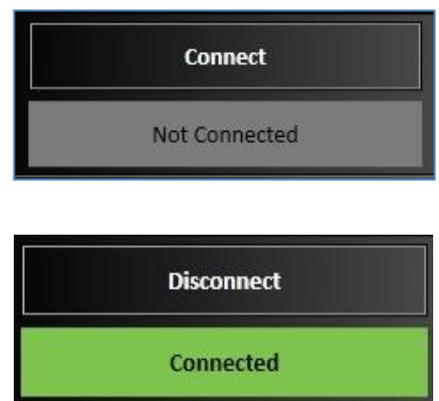
Once the USB firmware update is complete, Plasma5 CNC will connect to your signal generator by selecting *Connect* in the top left corner of the CNC window. When properly connected, the grey bar will turn green and display a *Connected* status. The tool is ready to be used.
